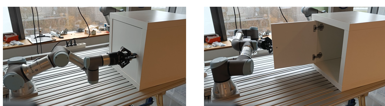
Using fixed grasps aggravates workspace constraints.
